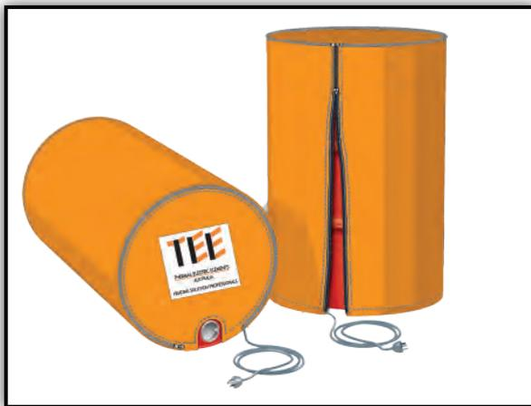
Thermal offers a simple, inexpensive and safe way to heat standard 205L (44 gallon) drums without having to build a hot room. Thermal's heater jacket zips up to form a miniature hot room around the drum and plugs into 240V power.
